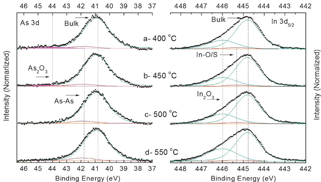
**Fig. 2.** As 3d and In 3d<sub>5/2</sub> XPS spectra of samples with postdeposition annealing temperature of (a) 400, (b) 450, (c) 500, and (d) 550 °C in forming gas for 5 min.
