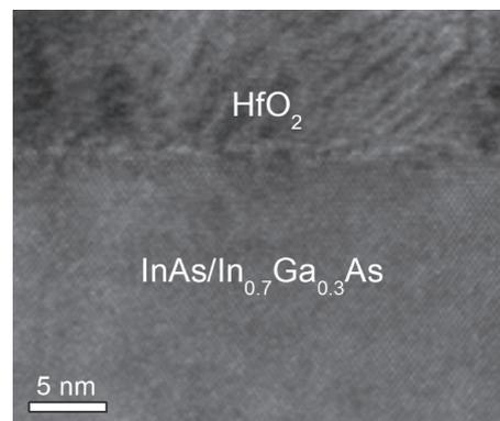
Fig. 1. Cross-sectional TEM image of the as deposited HfO<sub>2</sub>/n-InAs/InGaAs stacks.
