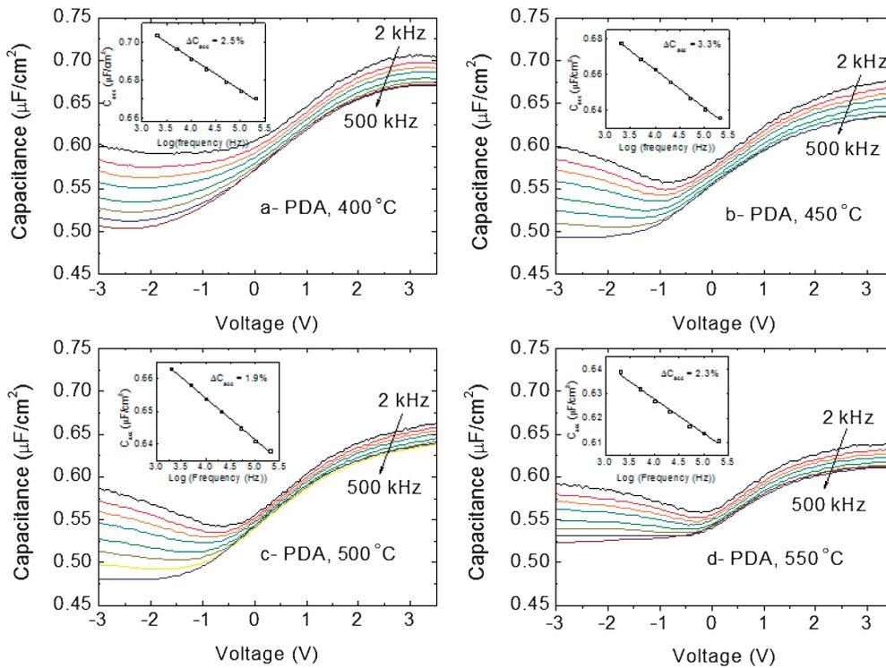
**Fig. 3.** Multifrequency  $C-V$  characteristics of  $\text{HfO}_2/\text{n-InAs}$  MOS capacitors with different PDA temperatures: (a) 400, (b) 450, (c) 500, and (d) 550 °C. The insets present the accumulation capacitance,  $C_{\text{acc}}$  vs measured frequency at a gate bias of 3.5 V.
