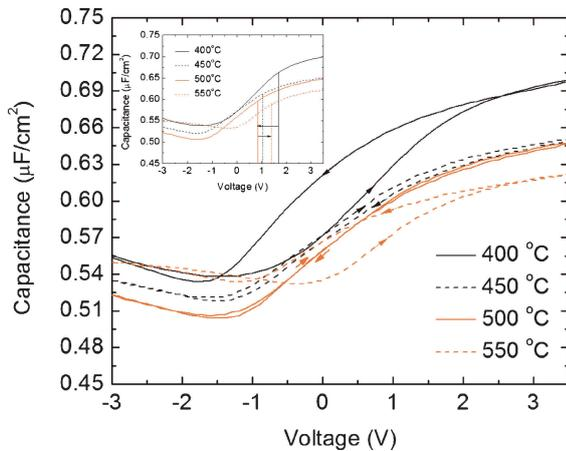
**Fig. 4.** Bidirectional  $C-V$  characteristics of samples measured at a frequency of 100 kHz. The inset of the figure shows the shift of the flat-band voltage with the PDA temperature.
